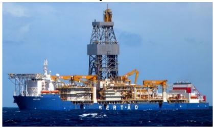
The drillship Sertão was delivered from Samsung Heavy Industries in 2012 and worked in Brazil for Petrobras until May 2015. It has been adapted for operating in High Pressure, High Temperature wells, and is capable of drilling wells up to 11,400 meters deep in depths of water of up to 3000 meters in pre-salt layer fields.
